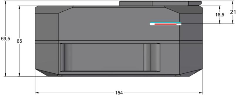
Figure 11: C3 camera head side view dimensions
