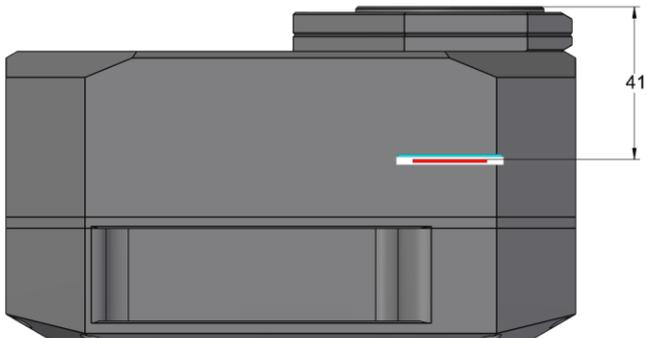
Figure 22: C3 camera with Internal Filter Wheel and “S” adapter base back focal distances with short M48 × 0.75 adapter
