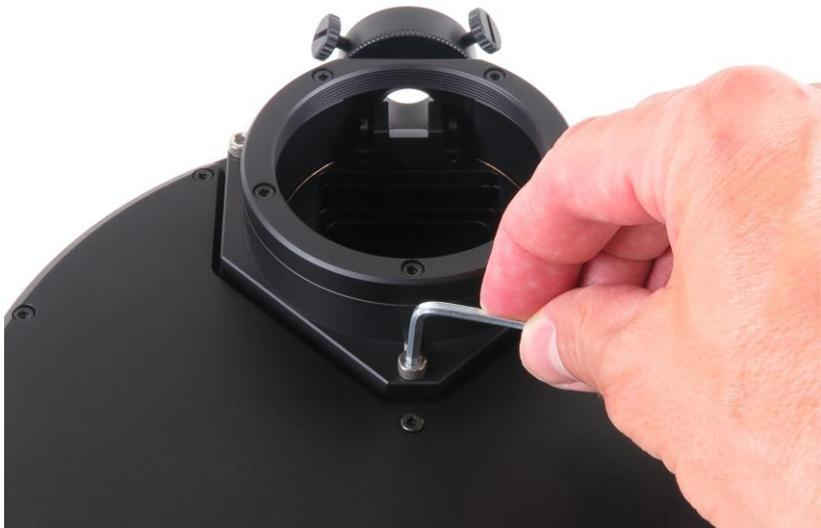
*Figure 41: Adjusting of the "pulling" screw*
