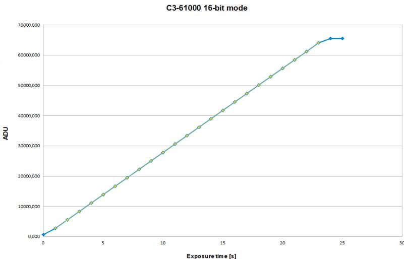
Figure 4: Response of IMX455 sensor in 16-bit mode
