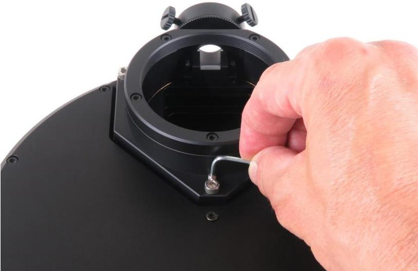
*Figure 40: Releasing of the “pushing” screw*
