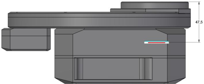
*Figure 26: C3 camera with “M” External Filter Wheel back focal distances with M68 × 1 version 1 adapter*
