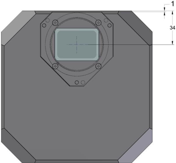
Figure 10: C3 camera head front view dimensions
