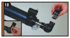
Insert the chrome barrel of the 20mm eyepiece into the diagonal and tighten the set screw.
