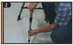
To set up the tripod, spread the legs outward until they are fully extended. Extend the center portion of each of the three tripod legs down 6-12".
