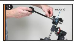
Slide the chrome end of the slow motion control cable onto declination axis gear shaft.
