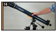
Place the telescope tube on the equatorial mount so that the tube is facing forward as pictured above.
