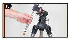
Tighten the threaded end of the counterweight bar into the declination axis of the equatorial mount.
