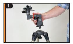
Locate the equatorial mount and place the base of the mount through the hole in the center of the tripod mounting platform.
