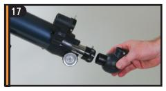
Insert the diagonal into the focuser and tighten the set screw.
