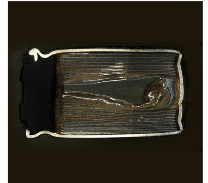
Foil capacitor, cut open, with dielectric in between; acquired with ZEISS Axio Zoom.V16, reproduction of object/camera 0.8
