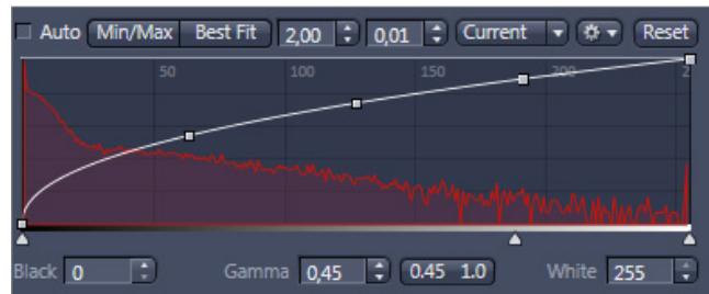
As seen here, a nonlinear Gamma curvature in the range of 0.45 over the whole dynamic range often delivers good results for transmitted light images.
