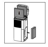
4 After the pre-filters are properly put back in the appliance, reset the filter lifetime counter. (Refer to chapter 7 "Resetting the filter lifetime counter".)
