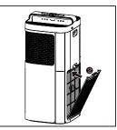
7 Repeat the above steps and assemble the air purification filter for the other side of the appliance. 8 Press both fasteners on left and right side of the top cover then lift the top cover to open it.
