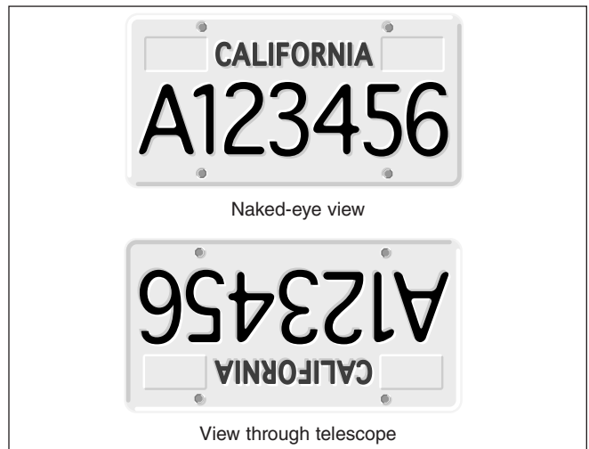
Figure 8. The view through a reflector telescope is rotated 180°
