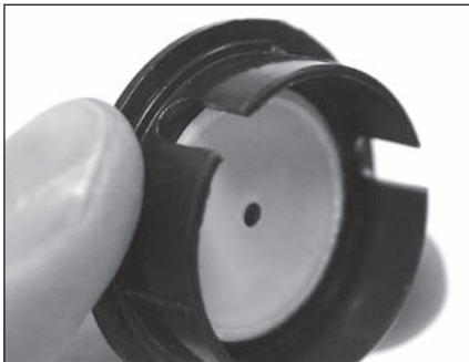
Figure 12. The quick collimation cap, which features a reflective inner surface, helps in centering reflections of the optics in the focuser during the collimation process.
