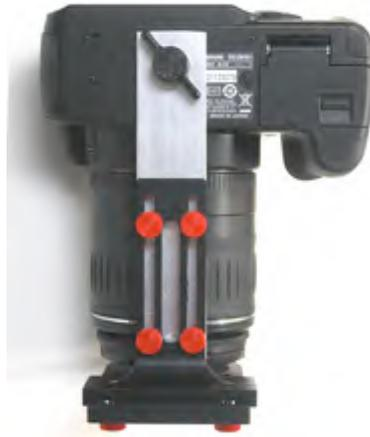
Below is the optical stack – eyepiece + RS-Spectroscopy + DSLR. Notice the orientation of the RS-Spectroscopy and the DSLR lets the RS-Spectroscopy disperse the spectrum along the long dimension of the DSLR sensor
