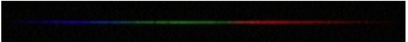
Some of the broad dark spectral features are visible. To make them more visible, the height of the spectrum can be stretched in Photoshop (image : image size) to stretch the spectral features into lines.
