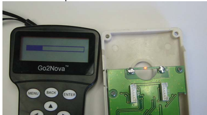
Figure 9. Adjust the LED brightness by a hand controller
