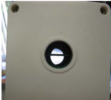
Figure 4. SmartEQ™ with integrated polar scope illumination LED
