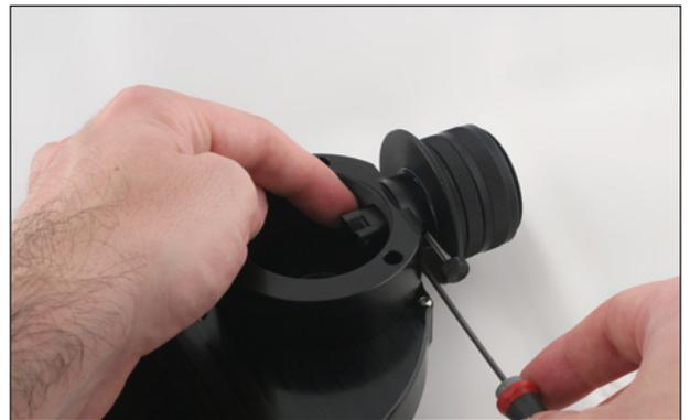
To adjust the pickup prism, you need to slightly undo the locking screw (the access hole is just below the locking screw), making sure that you undo it only "slightly". There's a captive recess that will prevent the prism support to falling, but this will not work if the screw is undone too much, causing the support to fall out of place.
