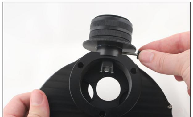
Simply adjust the focusing ring counter-clockwise, and the camera support will smoothly and precisely go up: turn clockwise, and it will go down. It's as easy as that! When focused, just tighten the locking ring slightly (don't over tighten!), so that the assembly keeps rock solid! There's a total travel of about 5mm which, in addition to the supplied rings, will be enough to make it easy to focus your guide camera.
