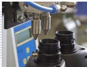
Fogging up or the formation of condensation inside the binoculars is totally prevented by this high-tech proprietary solution. Even temperature variations between  $-40^{\circ}\text{C}$  to  $+80^{\circ}\text{C}$  do not affect the functionality of STEINER nitrogen-filled binoculars. By 2-way-valve-technology, the maintenance of the binoculars is possible at any time even after many years.
