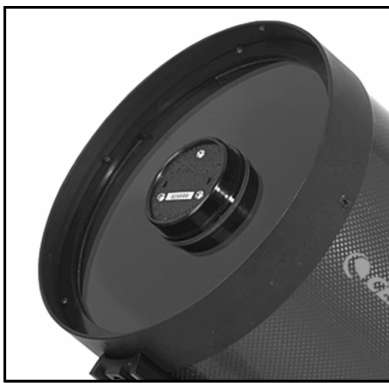
Figure 7-3 The three collimation screws are located on the front of the secondary mirror housing.
