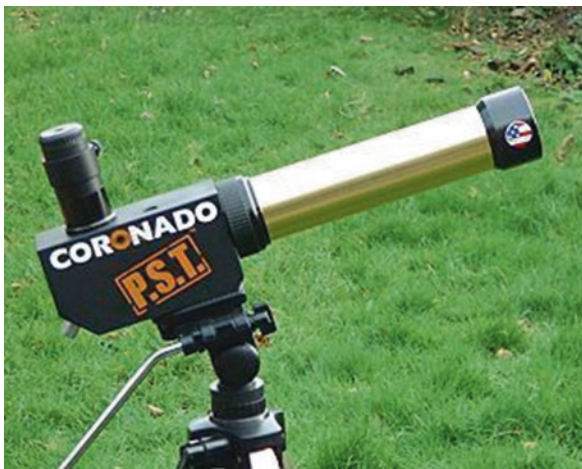
Fig. 2.14 A Coronado PST Hydrogen-Alpha telescope (Hands-on-Optics archive)
