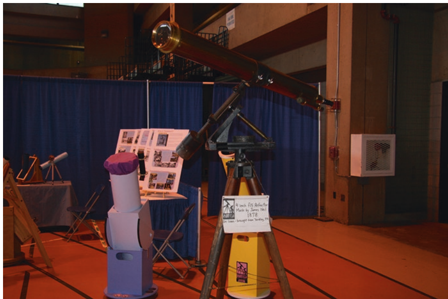
Fig. 2.10 A restored James Neil 4-inch f/15 refractor on display at NEAF 2016 (James Chen)
