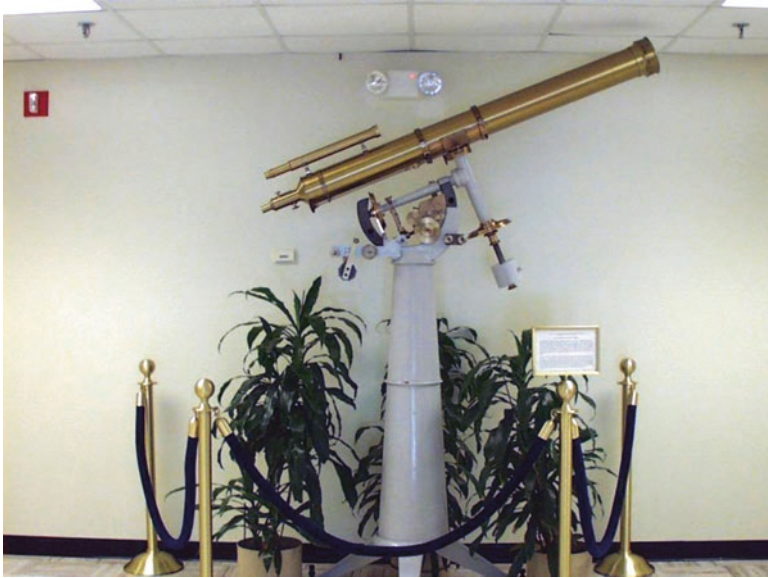
Fig. 2.9 A restored Alvan Clark 5-inch refractor at the U.S. Naval Observatory (USNO photo)
