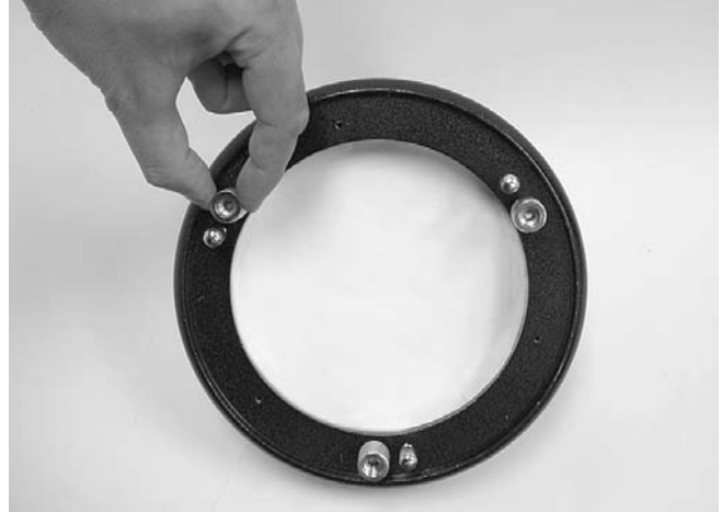
Figure 14: The tilt of the primary mirror is adjusted by turning one or more of the three larger thumbscrews.
