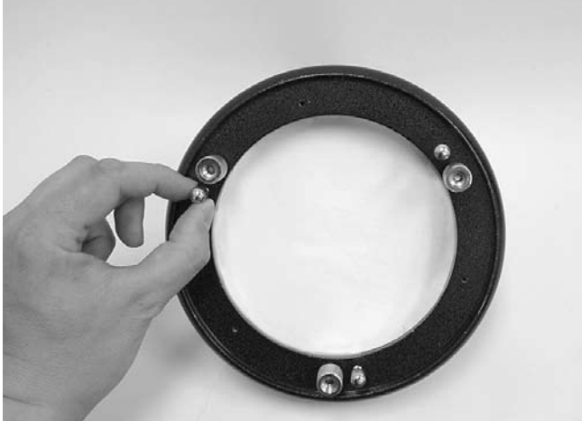
Figure 13: The three small thumbscrews that lock the primary mirror in place must first be loosened before any adjustments can be made. A flat head screwdriver may be used to loosen these screws.
